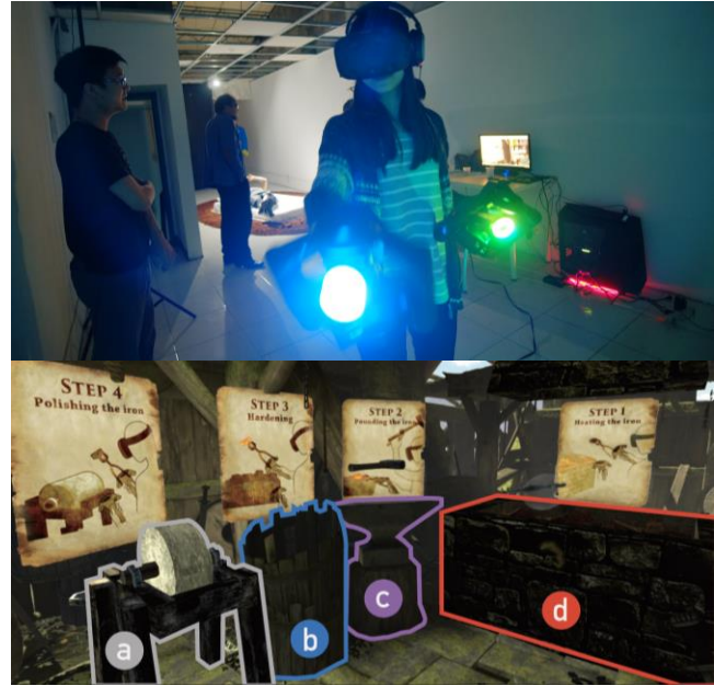
Figure 3: Learning the working process of blacksmith in the VR with controller-based haptic: (a) Vibration feedback, (b) Force feedback, (c) Wind feedback and (d) Heat feedback.
